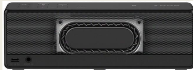
Fig. 7 Rear View with the Grille removed, showing the rear passive radiator
