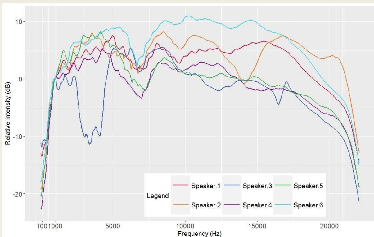
Figure 1: Frequency response of speakers anchored at 0dB at 1kHz
